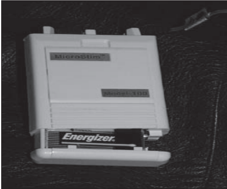
4.) Battery and Battery Compartment
